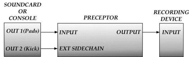
Very interesting sound effects can be achieved by doubling the same signal in the INPUT and in the EXT SIDECHAIN input with series equalizer connection. When You increase the level of selected frequencies, the *Preceptor* will react compressing them more than other frequencies and vice versa, when You decrease the level of selected frequencies, the *Preceptor* will not compress them. This technique can really improve the quality of your music. Keep experimenting!
