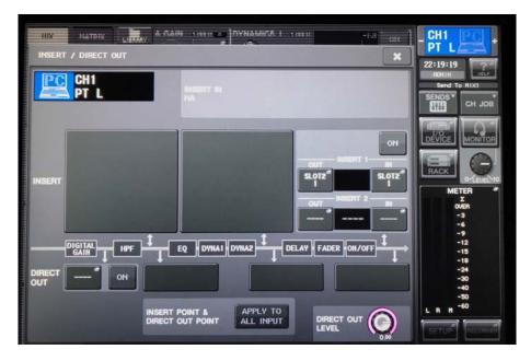
Figure 3-2 insert patch for the Dugan Speech System on a Yamaha digital mixer.
