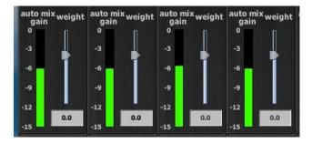
Figure 6-10 Multiple mic ambience: auto mix gain hovers around -9 dB for eight mics, -6 dB for four mics
