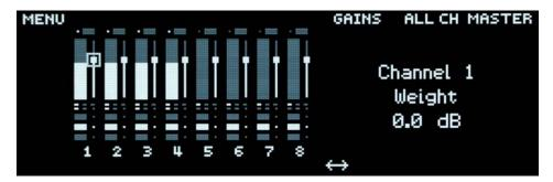
Figure 9-4 Altered Eight Channels screen clarifies how to navigate the controls
